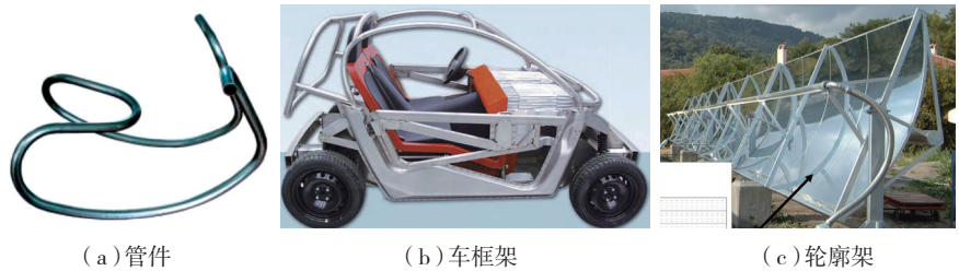
图10 德国蒂森克虏伯钢铁股份公司自由弯曲成形系统成形的复杂弯曲构件 Fig.10 Complex bending component formed by free bending system developed by Germany Thyssen Krupp Iron and Steel Company
